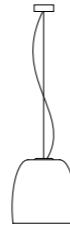
S5 Ceiling Rose Ø 120 mm Ceiling Rose LED Ø 160 mm H 45 mm Ceiling Rose LED DIMM Ø 200 mm H 45 mm Cable 2000 mm Diffuser Ø 360 mm H 365 mm
