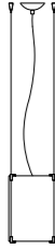
S1 Ceiling Rose Ø 120 mm Cable 2000 mm Diffuser Ø 240 mm H 330 mm
