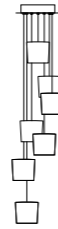
7R - 7S Ceiling Rose Ø 240 mm H 40 mm Cable 3000 mm Diffuser Ø 135 mm H 150 mm
